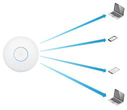
MU-MIMO with 1x1 clients: The UniFi HD AP communicates with four 1x1 clients at a time.
