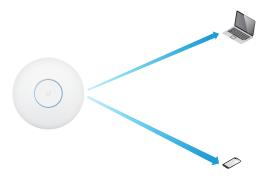
MU-MIMO with 3x3 and 1x1 clients: The UniFi HD AP communicates with one 3x3 client and one 1x1 client at a time.
