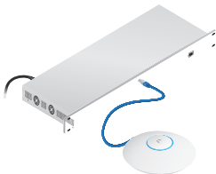
UniFi Switch with PoE Power Connection Diagram
